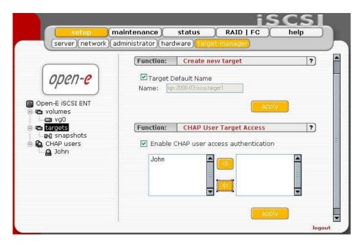
In this function you can create new targets, which will be seen in client stations as logical disks. You can change the name of any target.
